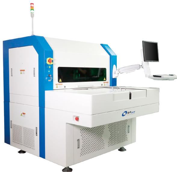
With fine focus of laser beam, the actual cutting gap can be as narrow as 10 microns, the removed material is less during processing, thus the depaneling is almost seamless and non-destructive. For the same size of raw materials, it wins more effective space with less material removal, save more material and reduce the total cost of the product.
